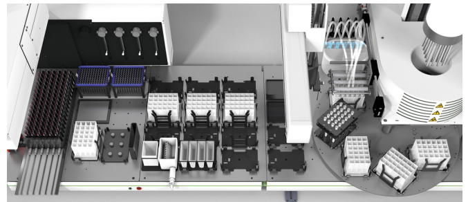
chemagic 360i Nucleic Acid Extractor integrated in PerkinElmer JANUS® Liquid Handling Workstation
