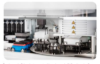
chemagic Prime instrument with a chemagic 360 unit and a Janus liquid handling unit for automated nucleic acid extraction and assay setup.
